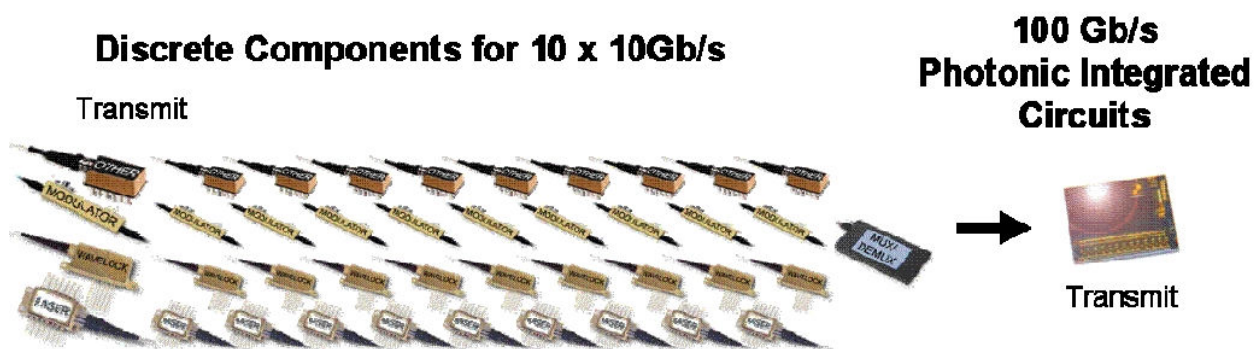
Figure A5-1 Infinera PIC Multiplexes and Transmits 10x10Gbps Wavelengths
