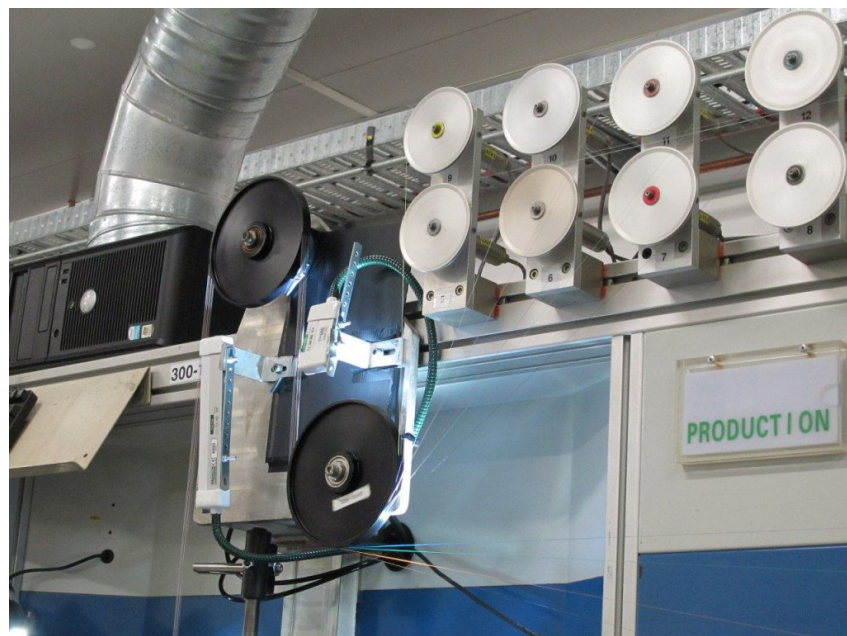
Combining Individual Colour-Coded Fibre Strands into 12-Fibre Ribbons
