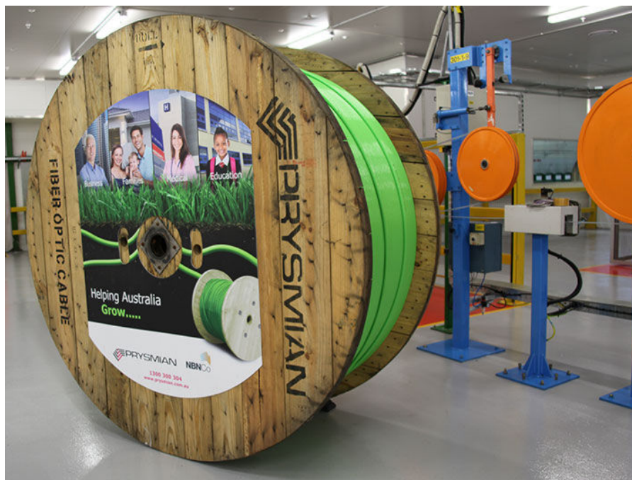
Finished 864-Fibre Distribution Cable on Drum
