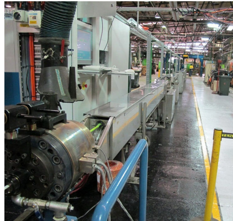
Applying NBN-Green Termite-Resistant Nylon Sheath
